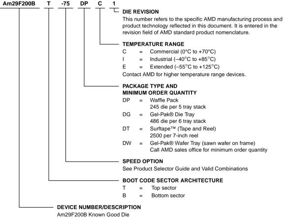
2 Megabit (256 K x 8-Bit/128 K x 16-Bit) CMOS Flash Memory—Die Revision 1 5.0 Volt-only Program and Erase
