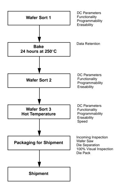
Figure 1. AMD KGD Product Test Flow
